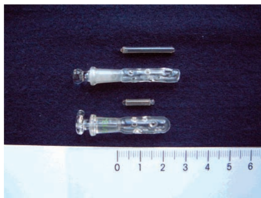
Figure 1. Perforated glass capsules for intraoral application of SBSE bars in BOSS analysis.
